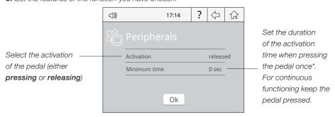
\*NB: The same can be applied inversely when continually pressing the pedal and releasing to activate.
