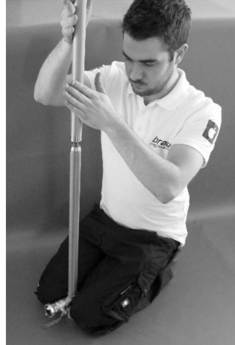
If you notice resistance when screwing in, do not use the open-end spanner to screw in the extension!
