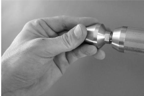
Place the retractor on the female thread of the outlet nozzle. Screw it in by hand carefully as far as it will go.
