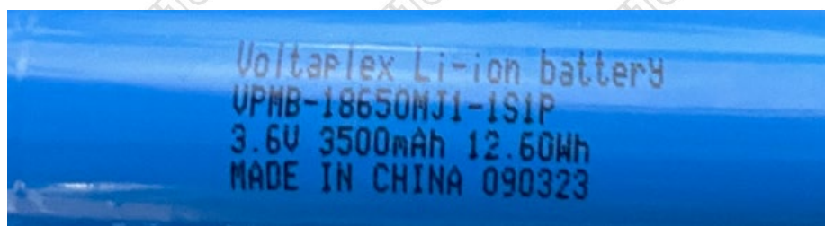
Figure 4 label of battery (标签图)
