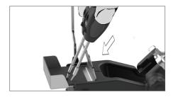
Lift up the Tweezer and press against the stand to insert the cartridge untill you reach the mark\*.
